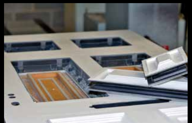
Door after routing operation
